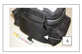
Soldering Iron – Pierce through the material and follow the outline of the large hole, letting the iron melt the material. Check the fit of the connector (large hole). Leave the connector in place & use the soldering iron tip to pierce the four holes.
