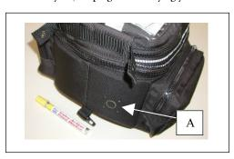
**Soldering Iron** – Pierce through the material and follow the outline of the large hole, letting the iron melt the material. Check the fit of the connector (large hole).
