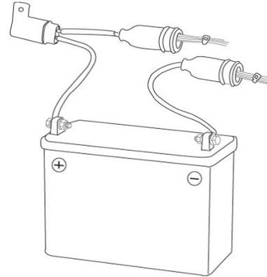
**STEP #3** – Attach the wires from all of the electrical devices to the terminal posts. Once wires are attached, slide the boot back over the terminals and zip tie the boot in place over all of your connections.
