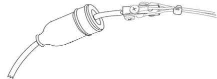
**STEP #4** – Install the 20 amp fuse into the fuse holder and tuck the fuse holder into a cavity near the battery and tie-wrap it to a stock wiring harness if possible.
