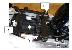
STEP #3 – Attach the bracket to the rear rearset-mounting lug [B]. Important: Only remove one rearset bolt at a time since the rearset bracket also supports the exhaust! The supplied spacer must be placed in the front hole to maintain proper alignment. Reinstall the rearset with the bracket & spacer sandwiched between the rearset & the frame. Re-use the stock bolts; tighten to the recommended torque.
