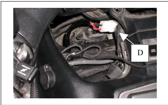
GL1500 Finished installation. Notice white "T" connector [D].
