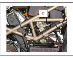
**STEP #4** - Apply the remaining ty-wraps in useful locations. Do NOT allow the harness to directly contact the motor or exhaust.
