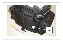
STEP #3 – Use either a soldering iron with a thin narrow tip or a hot knife & nail to cut the holes. Either will make the holes easily. The hot knife-edge (or iron) will cauterize the nylon, keeping it from fraying years later.
