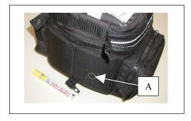
**STEP** #3 – Use either a soldering iron with a thin narrow tip or a hot knife & nail to cut the holes. Either will make the holes easily. The hot knife-edge (or iron) will cauterize the nylon, keeping it from fraying years later.
