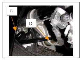
**STEP #3 - Do NOT allow the harness to directly contact the motor or exhaust.** Continue routing the harness between the frame and the motor. Follow the clutch hose out toward the bottom of the steering head tube [E]. Route the harness up into the steering head tube [D].
