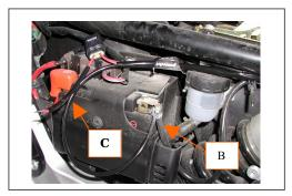
**STEP #2** – Remove negative battery lead [B]. Remove the positive battery lead. Slide the red cover off of the battery post [C]. Slide the cover back over both the stock wire and the fork terminal and attach the red wire. Reattach the battery negative lead. Run the wires down through the gap below the frame rails toward the front of the bike. Follow the very large wiring harness from under the seat toward he front of the bike.
