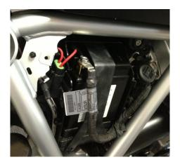
**STEP #2** – Stretch out the wiring harness. Grab the rubber boot (covering the white t-connector) end of the harness and start routing the harness from the right side near the battery to the left side passenger foot peg. Next remove the negative battery connection, followed by the positive battery connection. Connect the red & black wire as follows:
