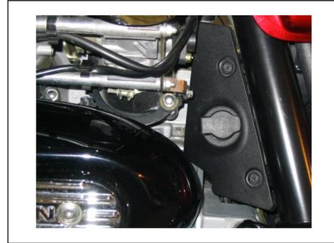
STEP #4 – Locate the plug for the socket which is taped to the harness with blue tape in the 1<sup>st</sup> photo fig.A. Attach the connector to the socket and test the socket for power.
