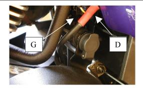
STEP #4 — Remove the top clutch cable mounting bracket bolt [E]. Loosen the ground lug [F] & remove the lower solenoid cable [D] to ease the installation. Slip the notch in the bracket over the lower clutch cable bracket bolt and align the bracket with the top hole. Add the supplied washer to the clutch bracket top bolt [E] & tighten the ground and clutch bracket bolts. Reinstall the solenoid cable [D].
