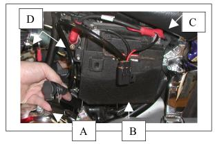
STEP #2 – Attach the white connector to the back of the Powerlet socket and slip on the black boot [A]. Install the fuse in the fuse-holder [B].
