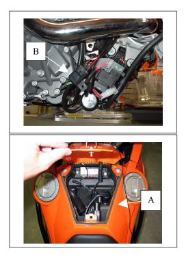
**STEP #3** – The center terminal is plus and the outer ring is negative (see dwg below). Apply either dielectric grease or Vaseline to the spade terminals. Connecting the white "T" will connect the red wire to the POSITIVE terminal and the black wire to the NEGATIVE terminal. Install the fuse in the fuse-holder. Use a voltmeter to check if the polarity is correct.
