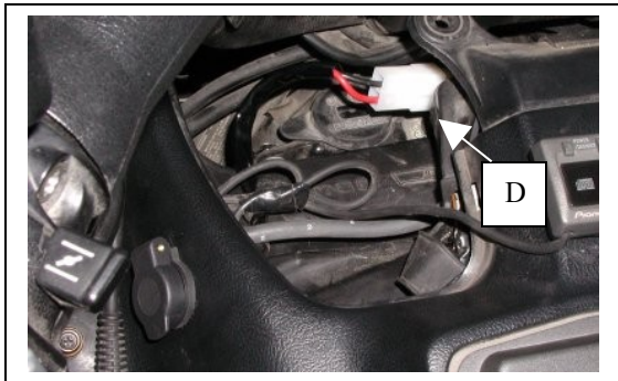
GL1500 Finished installation. Notice white "T" connector [D].
