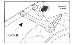
Many times the exhaust is hanging from the rearset and this can be heavier than expected. If your exhaust is hanging from the rearset, loosen both rearset bolts but do not remove them from the tail section sub-frame. By removing only one bolt at a time the weight of the exhaust will hang on the installed bolt. The bracket fits between the sub-frame and rearset and the supplied spacer [E] must be placed between the sub-frame and other rearset mounting point to maintain proper alignment.
