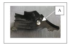
STEP #2 – Locate a suitable place on the panel to drill a 18mm hole (11/16" hole saw recommended and is available on our site). Do not use a flat wood drill [A]. A different finished location [E]. Watch the clearance behind the panel. The required clearance behind the panel is approx 1.5". Use a flat spot on the panel. Attach the socket to the panel; put a dab of Silicone on the socket and jam nut after assembly.
