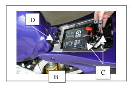
STEP #4 — Install the fuse in the fuse-holder. The center terminal is plus and the outer ring is negative (see dwg below). Apply either dielectric grease or Vaseline to the terminals. Connect the red wire to the POSITIVE terminal and the black wire to the NEGATIVE terminal. Install the fuse. Use a voltmeter to check if the polarity is correct.
