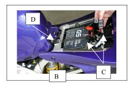
STEP #4 — Install the fuse in the fuse-holder. The center terminal is plus and the outer ring is negative (see dwg below). Apply either dielectric grease or Vaseline to the terminals. Connect the red wire to the POSITIVE terminal and the black wire to the NEGATIVE terminal. Install the fuse. Use a voltmeter to check if the polarity is correct.
