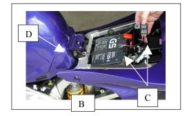
**STEP #3** – Install the fuse in the fuse-holder. The center terminal is plus and the outer ring is negative (see dwg below). Apply either dielectric grease or Vaseline to the terminals. Connect the red wire to the POSITIVE terminal and the black wire to the NEGATIVE terminal. Install the fuse. Use a voltmeter to check if the polarity is correct.
