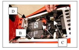
**STEP #3** – Install the fuse in the fuse-holder. Next attach the spade connectors to the socket. The center terminal of the Powerlet socket is plus and the outer ring is negative (see dwg below). Apply either dielectric grease or Vaseline to the terminals. The boot on the back of the socket are oriented so the wiring harness will route straight up from the socket, hiding it under the tail fairing.
