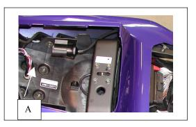
STEP #3 – Select a route for the harness. Follow stock wiring harnesses where possible. Do not allow the harness to contact the motor or exhaust. Tywrap the harness in place.
