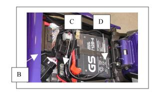
STEP #4 – Locate a suitable chassis ground point. In this example we used the gas tank bolt. If a chassis ground cannot be located, use the battery negative post. Connect the terminals as follows:
