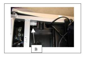
STEP #4 – The center terminal is plus and the outer ring is negative (see dwg below). Use a voltmeter to check if the polarity is correct.
