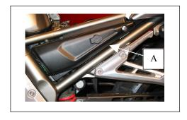
STEP #2 — Drill a 18mm hole into the panel (11/16" hole saw recommended and is available on our site). This hole must be drilled in about the same spot as shown [A]. Watch the clearance behind the panel; make sure the socket has room. If the hole is too small for the socket open it with emery cloth or a file. Attach the socket to the panel; use a dab of silicone on the socket and jam nut.
