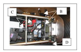
STEP #4 — Install the fuse in the fuse-holder. The center terminal is plus and the outer ring is negative (see dwg below). Apply either dielectric grease or Vaseline to the terminals. Connect the red wire to the POSITIVE terminal and the black wire to the NEGATIVE terminal. Use a voltmeter to check if the polarity is correct.
