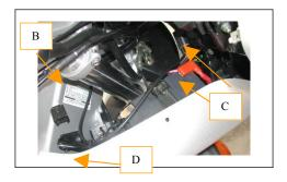
Pull most of the harness through the hole toward the engine (under the tank). Next **remove the negative battery connection**. Loosen the positive battery connection. Slip the red wire under the red battery boot [C]. You may need to trim the red boot to accommodate the added wire.
