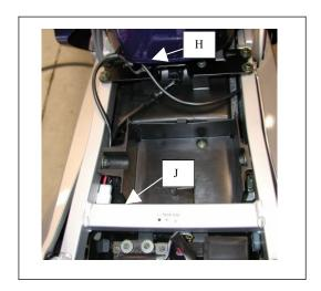
STEP #3 – Adjust the slack in each section, tighten ty-wraps.
