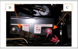
STEP #4 – Install the fuse in the fuse-holder. The center terminal is plus and the outer ring is negative (see dwg below). Attach the wires to the socket. Apply either dielectric grease or Vaseline to the spade terminals. Connect the red wire to the positive spade terminal & the black wire to the negative terminal. Use a voltmeter to check if the polarity is correct.
