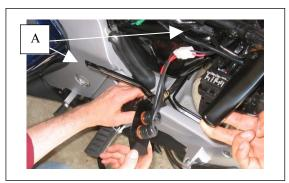
STEP #2 – Stretch out the wiring harness. Using a ty-wrap, attach the fuse holder to the stock vehicle wiring harness [D] located on the right side of the battery. Next remove the negative battery connection, followed by the positive battery connection. Slip the red wire under the red battery boot [C]. You may need to trim the red boot to accommodate the added wire. Connect the red wire to the battery posts as follows:
