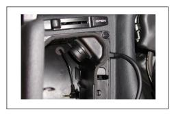
STEP #3 – Attach the socket to the panel. Use a dab of Silicone on the socket and jam nut after assembly. Do not use Loctite or over-tighten.
