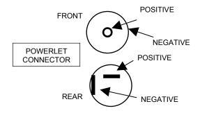
STEP #5 — Use a voltmeter to check if the polarity is correct. Replace the pocket. Enjoy!
