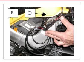
STEP #3 - Apply the two ty-wraps. Use one to secure the fuse-holder and the other near point [E]. Do NOT allow the harness to directly contact the motor or exhaust. Continue routing the harness between the frame and the motor. Follow the clutch hose out toward the bottom of the steering head tube [F]. Route the harness up into the steering head tube. Attach the black wire to the radiator mounting bolt [G] or other chassis bolt in the area.
