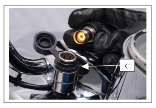
STEP #5 - Do NOT allow the harness to directly contact the motor or exhaust.
